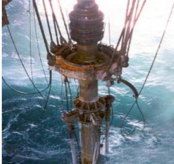
**Figura 2.20.** Conductor Marino (Riser).
