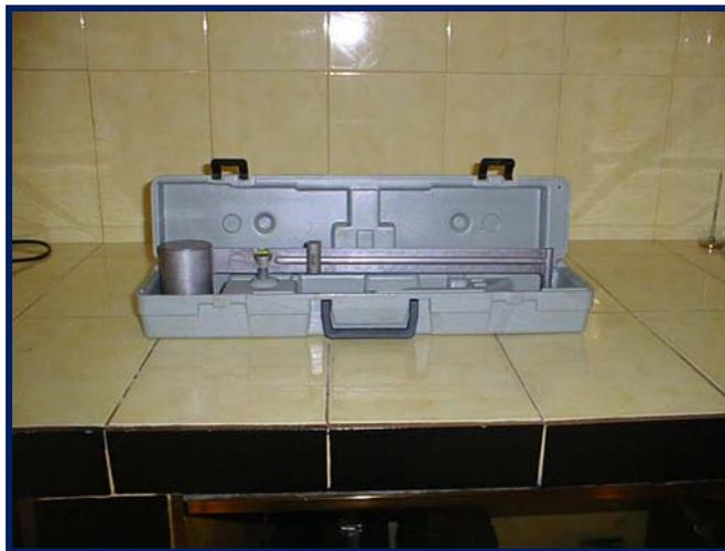
FIGURA A-2: BALANZA PARA LODOS
