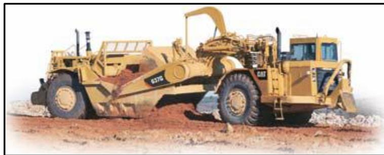
*Figura 3.1 Mototraíllas (Wheel Tractors Scrapers). Cat® Product Line Brochure (2010)*
