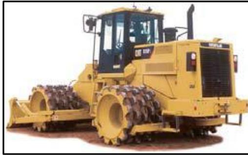
*Figura 3.7 Compactadoras Pata de Cabra (Soil Compactors). Cat® Product Line Brochure (2010)*
