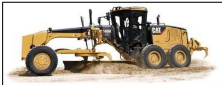
*Figura 3.9 Motoniveladora (Motor Graders). Cat® Product Line Brochure (2010)*
