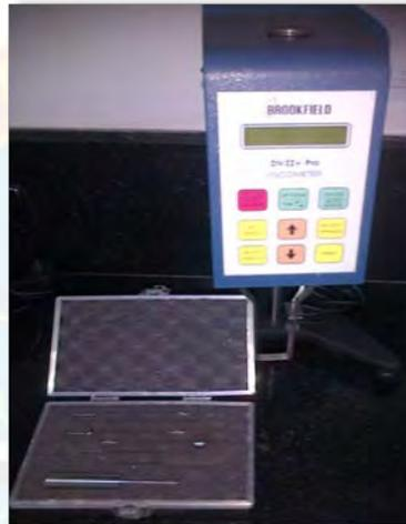
**Figura B.3.4 Viscosímetro digital Brookfield DV-II+ Pro.**
