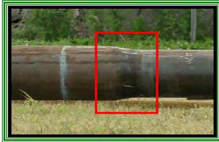
**Figura 2.6 Junta roscada expansible.**
