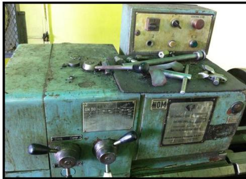
**Figura 4.25 Cabezal**
