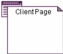
A UML class diagram for 'ClientPage'. It is represented as a rectangle with a folded top-right corner. A small icon of a web browser window is positioned at the top-left corner of the rectangle. The text 'ClientPage' is centered within the rectangle. | Las páginas del cliente tienen métodos que se ejecutan solamente del lado del cliente, como por ejemplo, Java Applets y controles ActiveX. |
