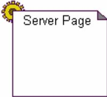
A UML class diagram for 'Server Page'. It is represented as a rectangle with a folded top-right corner. A yellow gear icon is positioned at the top-left corner of the rectangle. The text 'Server Page' is centered within the rectangle.                 | Los scripts de las páginas del servidor representan los métodos de esta clase. Las páginas del servidor crean las páginas del cliente.     |
