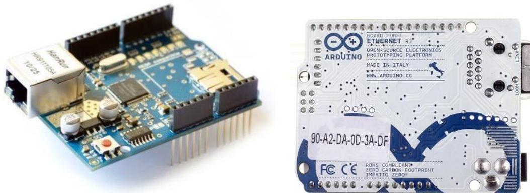
Figura 16. Arduino Ethernet Shield
