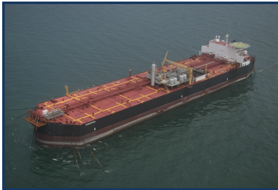
Figura 2.6 FSO (Floating Storage Offloading) Nabarima [8].
