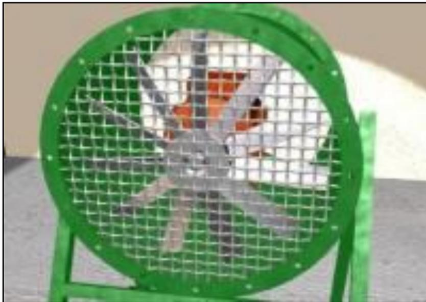
Figura 5.35 Ventilador industrial turboaxial transportable
